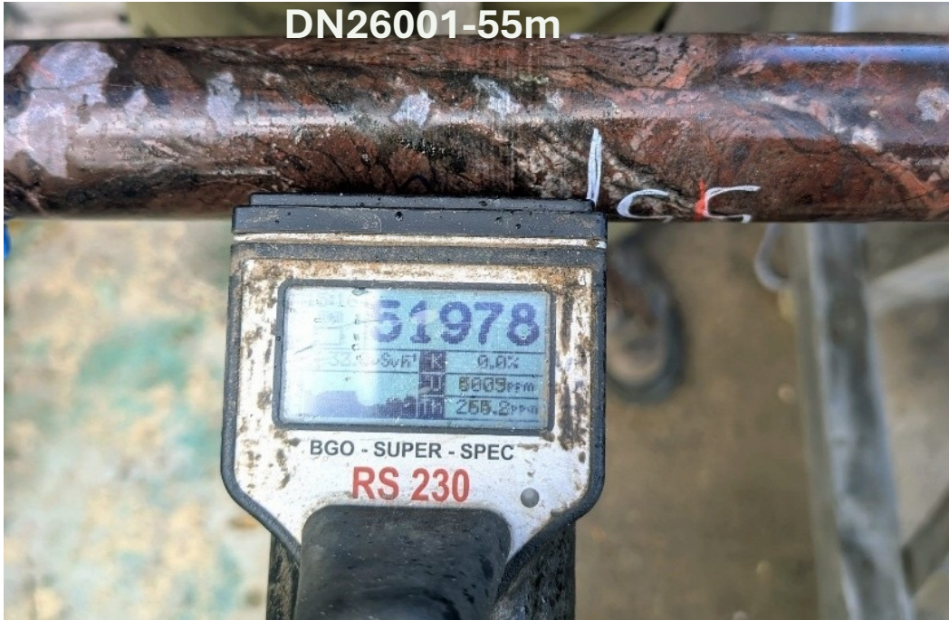
DN26001-55m Mineralized Psammite / Gabbroic Contact. Uranium mineralization hosted in fractures/veinlets associated with intense hematite and silica alteration.
